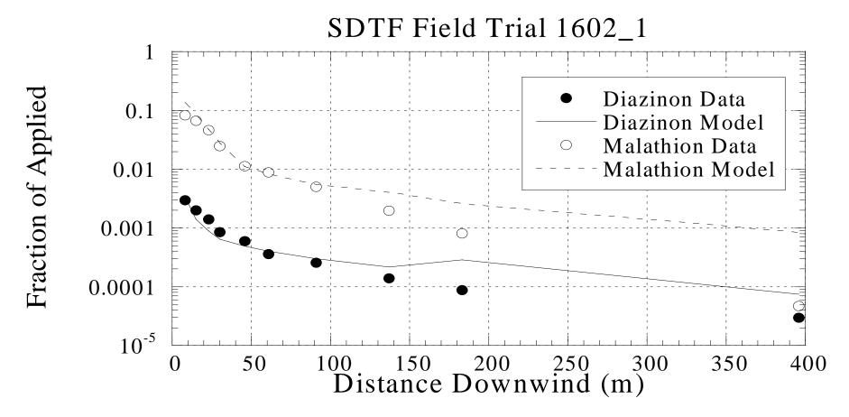
Lowest ambient temperature (6.7°C): Diazinon (8004,  $D_{V0.5} = 312$  µm), Malathion (TX-6,  $D_{V0.5} = 162$  µm)
